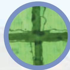
Back-side chipping after the standard step-cut process
