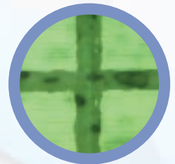
Back-side chipping after scribe and dice process
