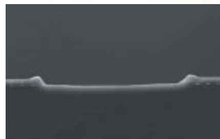
This SEM image shows a cross section of an IC wafer after laser scribing with NextStep. The image shows the clean trench left by the CO 2 laser
