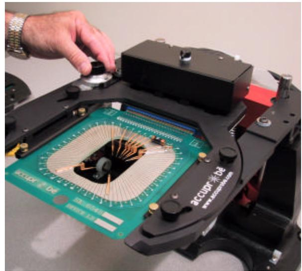
ient, repeatable and fast way to setup theta adjustment for each card. The Position Saver allows a very fast card changeover cycle because individual card assemblies can be identified with a specific theta reference number. Each subsequent use of a specific probe card can then be setup quickly by inserting the card and simply dialing in the saved position number to achieve the proper theta alignment.
