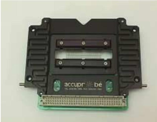
Probe Card assemblies are available for the GSI-724 and 770 Laser trim systems. Laser Trim probe cards are offered for 1206, 0805, 0603 and 0402 chip formats. Other chip formats can be accommodated on a custom basis. These probe card assemblies utilize Accuprobe's Probe Ring style epoxy probe arrays or traditional metal blade probes, and the entire probe fixture concept has been separated into three modules for easy repair and replacement and to minimize cost for the laser trim operation.
