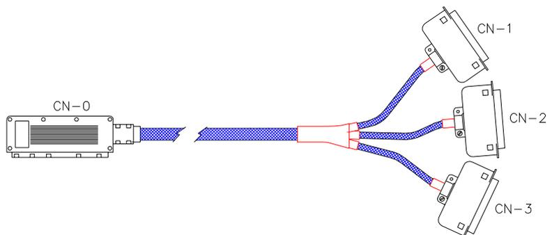
The measurement system interface from the probe card utilizes a standard 96 pin DIN connector and is connected to the measurement system with standard Cinch 48 pin connectors. Interface cables can be assembled by the user or can be ordered complete as shown below.
